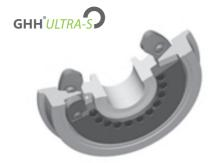
**GHHULTRA-5°** is the new flagship product among the high-elastomer wheels. Thanks to the innovative design of the rubber segments, it is possible to combine low radial stiffness (20 to 40 kN/mm) with a high wheelset load of up to 12.5 tons. The running circle is 600 mm when new and 520 mm when worn.
